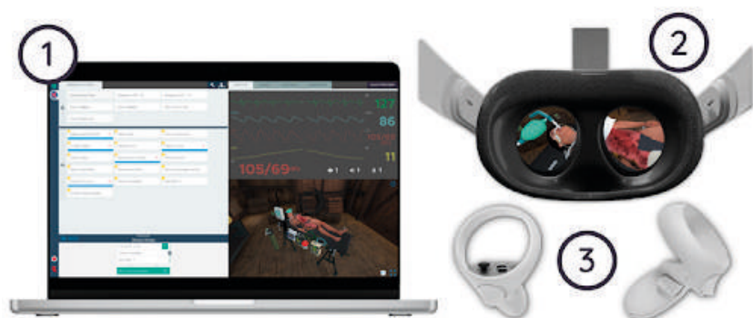
Immersive VR training setup allows for a lightweight, high-fidelity simulation consisting of (1) Facilitator PC (2) VR headset(s) and (3) hand controllers. Source: SimX Inc.
